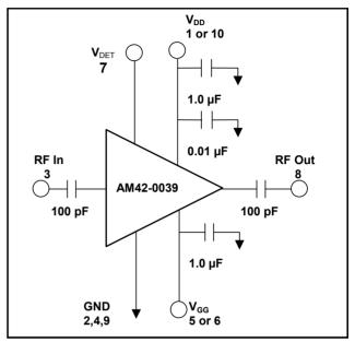
4. Apply -2 volts to pin 5 or 6 (V<sub>GG</sub>), prior to applying +8 volts to pins 1 or 10 (V<sub>DD</sub>). Adjust V<sub>GG</sub> for typical drain current.
