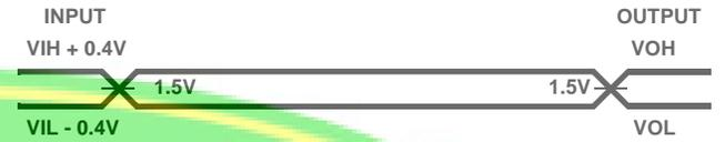
AC Testing: All AC Parameters tested as per test circuits. Input RISE and FALL times are driven at 1ns/V.
