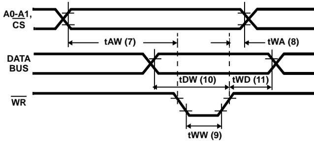
FIGURE 30. WRITE TIMING
